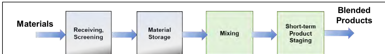
Figure 5. Blended products flow diagram: screened (No waste material is generated other than plastic bags from bagged feedstock, screened oversize is used for other products)
